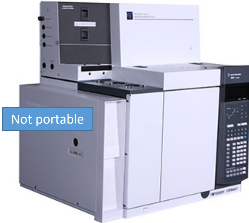
Example Wasson Gas Chromatograph like what PFT Technology Uses
